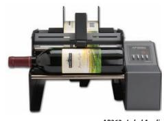
AP362e Label Applicator – applies labels automatically to round/cylindrical containers when the foot pedal is pressed.
